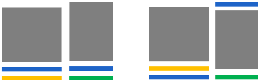
Figure 4.12: Example of both cases of the swap rail action; The left cell swaps the two rails and the right cell changes the position of the blue rail.
