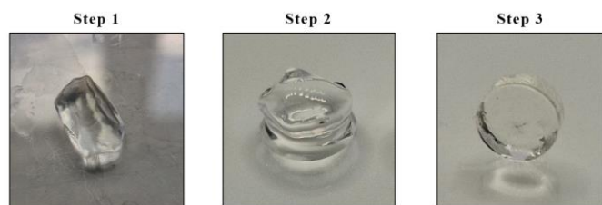
Figure 7 Dose optimization for GelNB-GelSH 5eq 10%. Step 1 is under-polymerized; Step 2 is over polymerized; Step 3 is printed with
