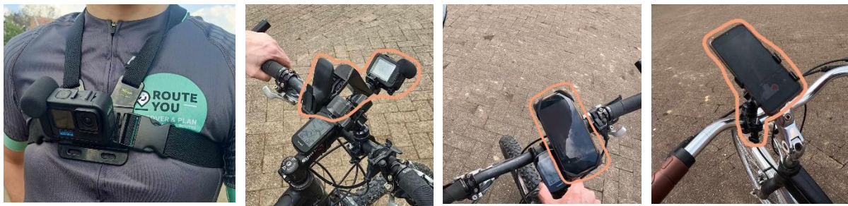
Figure 10 Different ways of mounting a recording device data collection while cycling, from left to right: GoPro on chest mount, GoPro mounted with an arm, Phone on a flat bike mount and Phone on a bike mount an with arm
