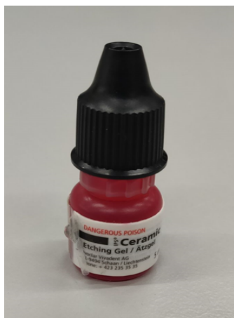
Foto 3: IPS ceramic etching gel 5% HF (Ivoclar Vivadent)
