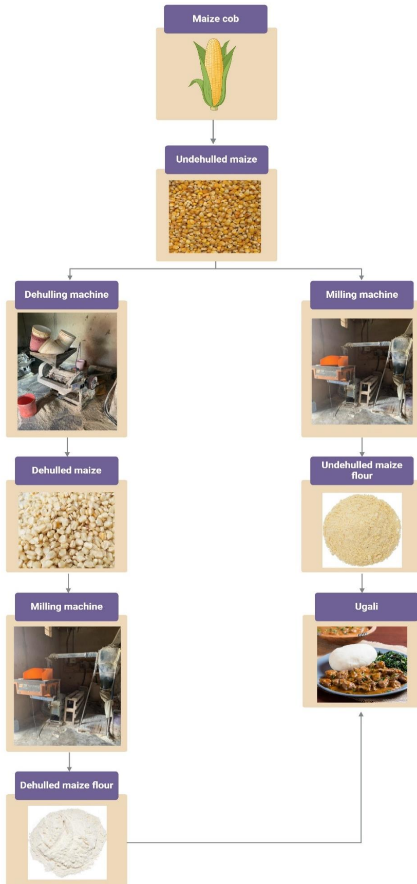
Figure 1.4. The process of going from maize to maize flour and to Ugali, from both undehulled and dehulled maize flour. This includes dehulling of the maize and milling of the maize flour.
