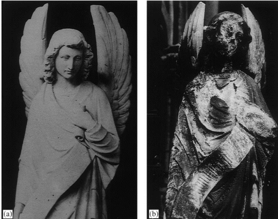
Figure 1: Images showing the effect of biodeterioration on an angel statue from the cathedral of Cologne, (a) shows the statue in 1880, (b) shows the statue in 1993 (Warscheid & Braams, 2000).
