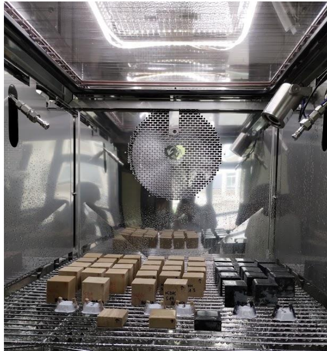
Figure 13: Image showing the position of the samples in the climatic chamber, the installed light strips can be seen at the top of the image.
