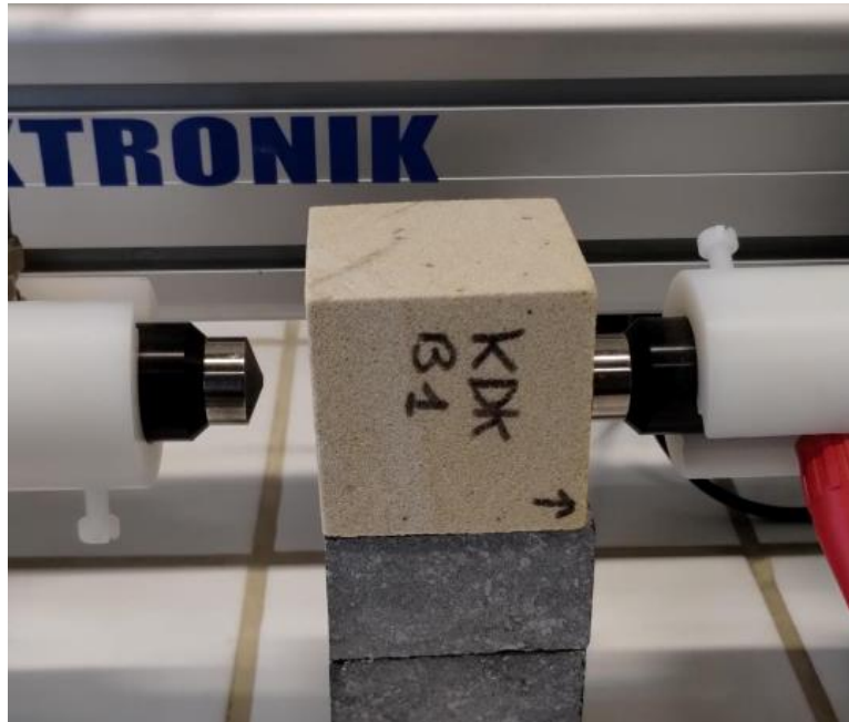
Figure 7: Image showing the orientation used for the UPV measurements, the two transducers that send out the waves can also be seen next to the sample.
