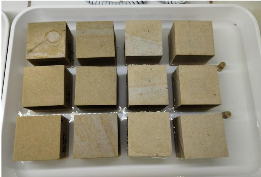
Figure 12: Example of one of the dishes used in the lab setup, these are the Bentheimer samples a couple of days after inoculation.
