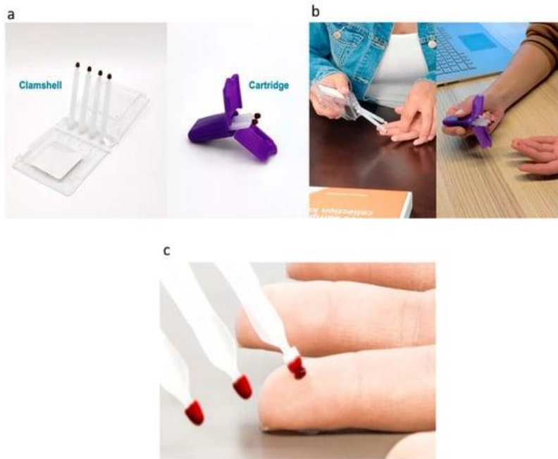
Figure 4: VAMS procedure: (a) VAMS tips are attached to a clamshell or cartridge; (b) tips are held at an angle to the blood, then removed after they are completely filled; (c) closeup of the blood absorption. ( https://www.mdpi.com/2218-1989/13/10/1038 )
