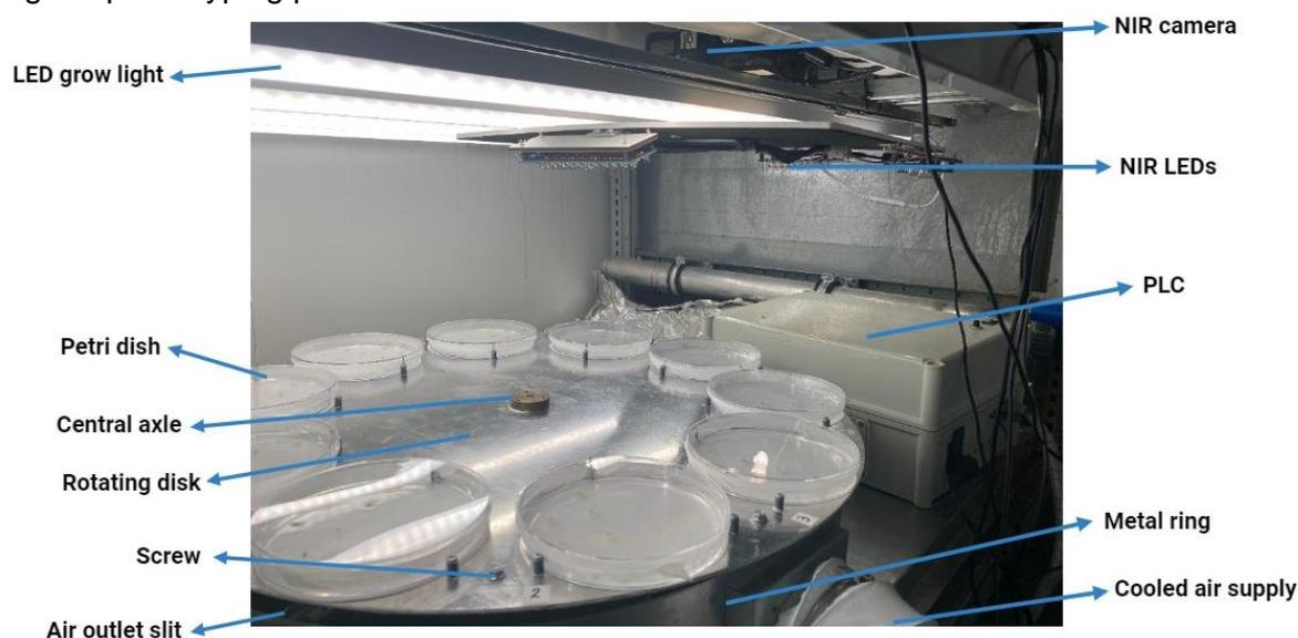
Figure 11. IGIS platform general setup. PLC: Programmable logic controller. LED: Light emitting diodes. NIR: near infrared. Figure by author using Biorender.
