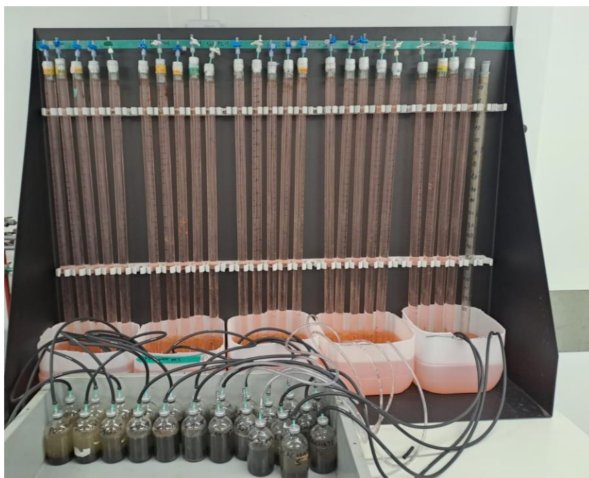
Figure 8: Set-up for conducting biochemical methane potential tests for six treatments (aquaculture solids from freshwater aquaculture, aquaculture solids at sea salt concentrations of 12 g/L, 20 g/L, and 35 g/L, and leachate in total and soluble forms), each executed in biological triplicates.
