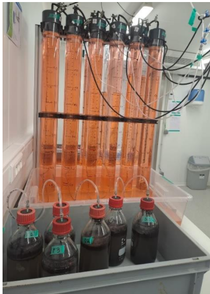
Figure 7: Left: Nine fed-batch reactors, with six reactors visible in the forefront and three additional reactors positioned behind the gas collection tubes. Three different treatments were performed, each in biological triplicates (aquaculture solids from freshwater aquaculture, aquaculture solids from saltwater aquaculture at concentrations of 12 g/L and a mixture of leachate and BSFL frass). Right: Schematic overview of the experimental set-up of one reactor.
