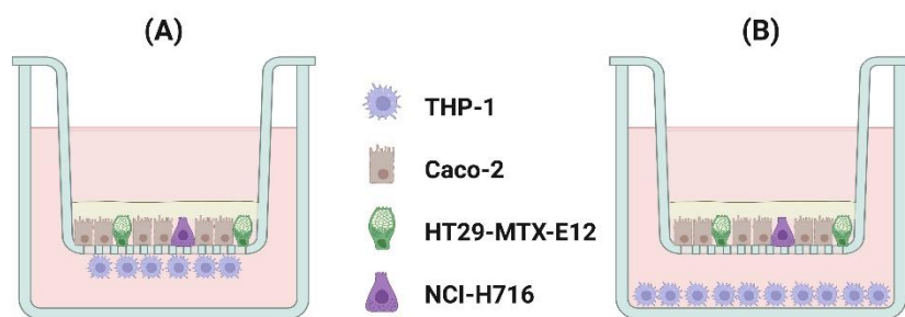
Figure 9: Visualization of two set-ups for the inclusion of macrophages in the triple model. (A) THP 1 cells are seeded at the basal side of a Transwell insert. (B) THP-1 cells are seeded at the bottom of a well-plate. Figure created with BioRender.com.
