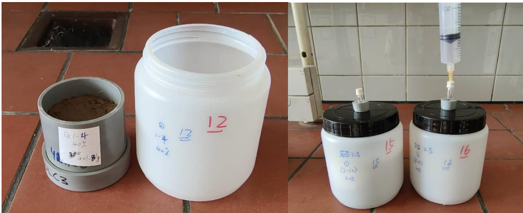
Fig. 6 Configuration for headspace CO 2 measurement – grey tube (Left) containing soil sample, larger white PE pots outfitted with a septum (left) in which the soil cores were periodically placed for measuring headspace CO 2 buildup and gas sampling with the a syringe (right)
