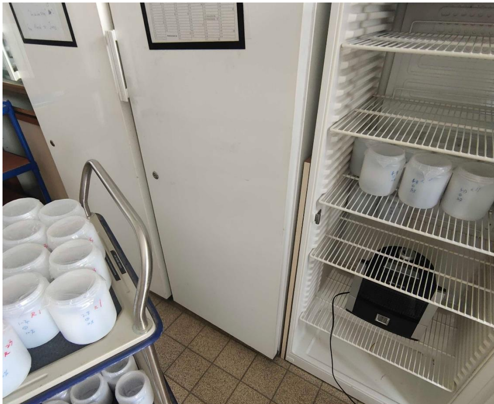
Fig. 5 Incubation Cupboard Setup with Soil Cores and Air Humidifier
