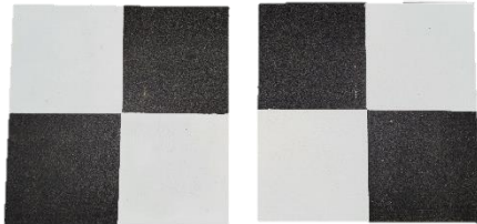
Figure 2: (Ground) control points made of bitumen
