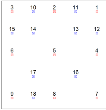
Figure 3: Ideal location GCPs (red) and CPs (blue)
