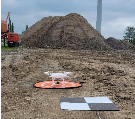
Figure 4: Land and take-off setup together with control point
