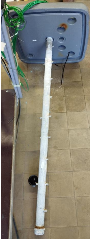
Figure 38: Thermocouples in lid of tank.
