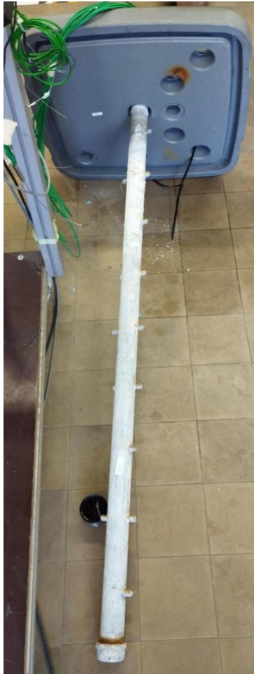
Figure 42: Thermocouples in lid of tank.
