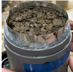
Figure 6: PVC tube to determine \mu of cork
