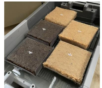
Figure 4: Set-up to determine the water absorption coefficient A_w
