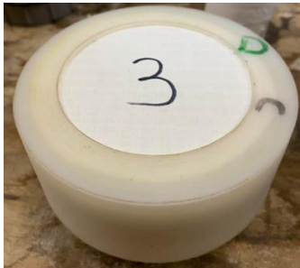
Figure 7: Plastic cup to determine \mu of magnesium oxide boards
