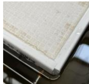
Figure 3: Magnesium oxide board with plastic U-profiles
