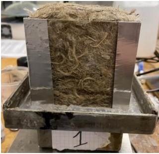
Figure 5: Metal cup to determine \mu of wood wool, cotton, grass and hemp
