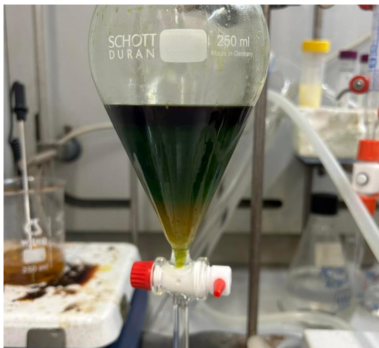
Figure 4.1: Presence of solid particles complicating the separation of the Ethyl acetate layer (upper layer) from the water layer (bottom layer)
