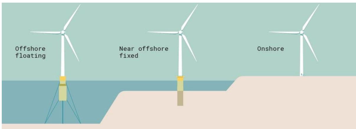
Figure 2 Representation of onshore, offshore fixed and offshore floating WT [19].
