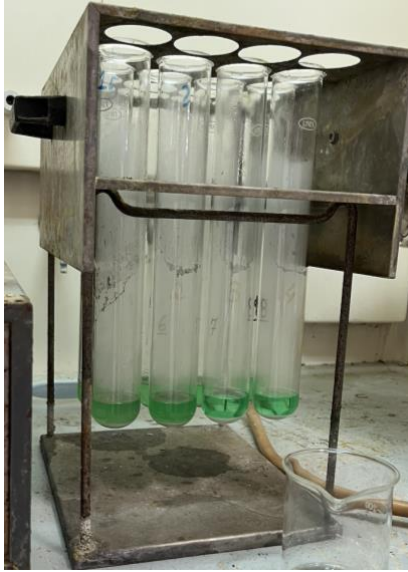
Figure 12: Illustration of the digestion of normal substrate for which the reaction ended since the solution is green and translucent.
