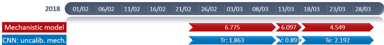
Figure F.7: Timeline with the RMSE per time period (Tr=train, V=validation, Te=test) used to develop a CNN hybrid model trained on the uncalibrated mechanistic model residual for effluent TSS, compared to the RMSE of the mechanistic model in these periods.
