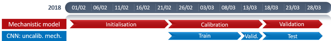
Figure F.4: Timeline with the time periods used to develop a CNN hybrid model trained on the uncalibrated mechanistic model residual for effluent TSS.
