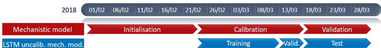
Figure E.1: Timeline with the time periods used to develop a LSTM hybrid model trained on the uncalibrated mechanistic model residual for effluent nitrate.
