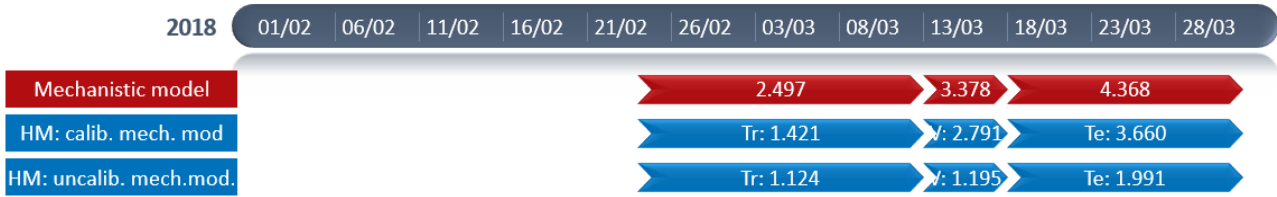
Figure 5.10: Timeline with RMSE per time period (Tr=train, V=validation, Te=test) used to develop a CNN hybrid model trained on the calibrated mechanistic model residual and a CNN hybrid model trained on the uncalibrated mechanistic model residual for effluent nitrate, compared to the RMSE of the mechanistic model in these periods.
