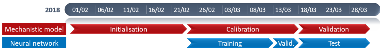
Figure 5.21: Timeline with the time periods used to develop a serial hybrid model in the first approach.
