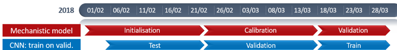
Figure 5.15: Timeline with the time periods used to develop a CNN hybrid model for effluent TSS.
