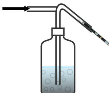
Figure 13: Sampling technique: VOC measurement in water using a washing bottle.
