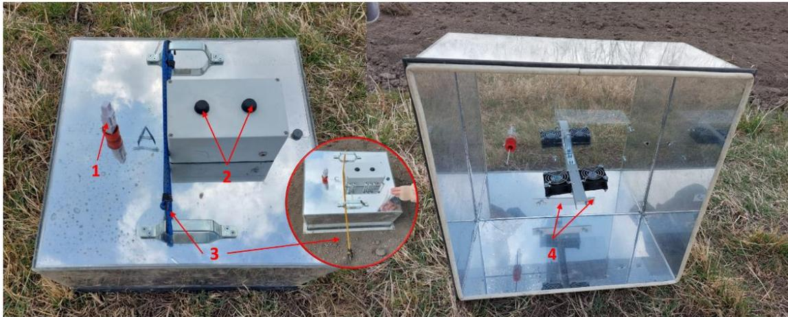
1. **Thermometer** measures headspace temperature
