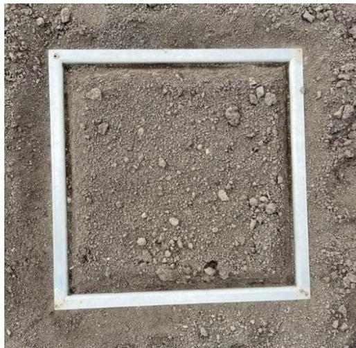
Figure 5. Stainless steel frame prepared for soil GHGs measurement in study field. Frames are used to keep gas-tightness (Butterbach-Bahl, Kiese, and Liu 2011).
