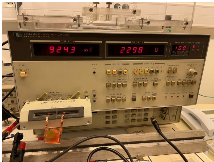
Figure 4- 23 LCR meter Measurement result of the sample without mirror
