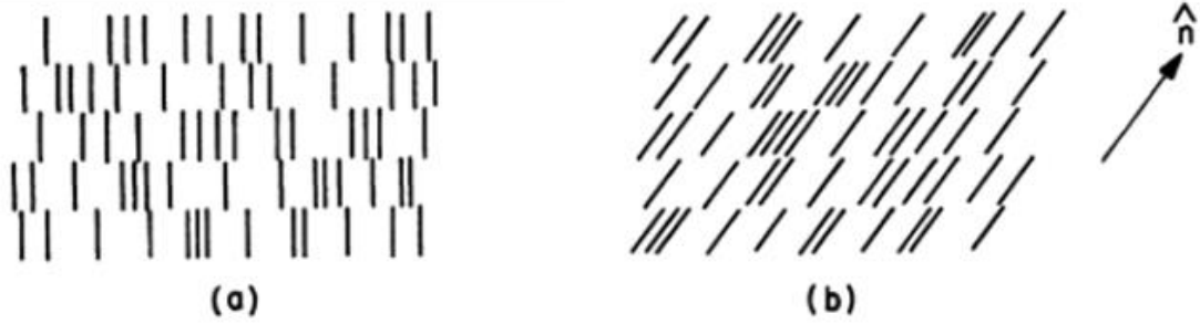
Figure1- 3 Schematic arrangement of (a) smectic A and (b) smectic C[5]
