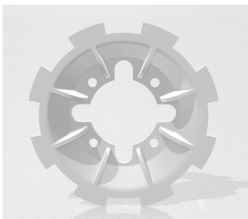
Figure 3.18: 3D model of the disc that is mounted on the rotating shaft. The outer part has eight openings to imitate a machine with eight pole pairs. Design of the disc done by Prof. Dr. Ir. Hendrik Vansompel
