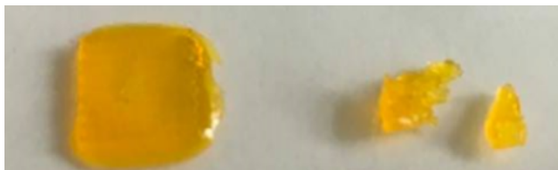
Figure 3.27: DLP printed scaffolds of PLA6AUP(3) (left) and PLA13AUP(3) (right) with an intensity of 19.51 mW/cm^2 , exposure time of 20 seconds, 1.5 wt% TPO-L and molar ratio PB/PI of 0.1
