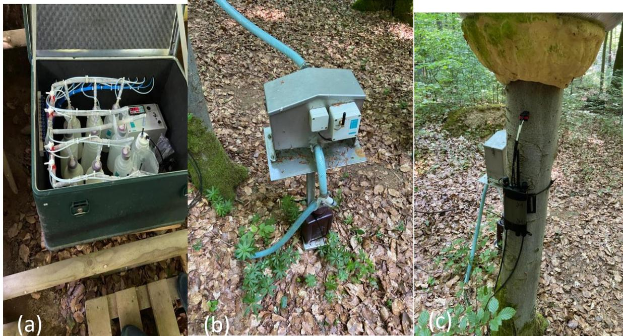
**Figure 3.** PE bottles for soil solution collection (a), throughfall measurement and collection, and stemflow measurements
