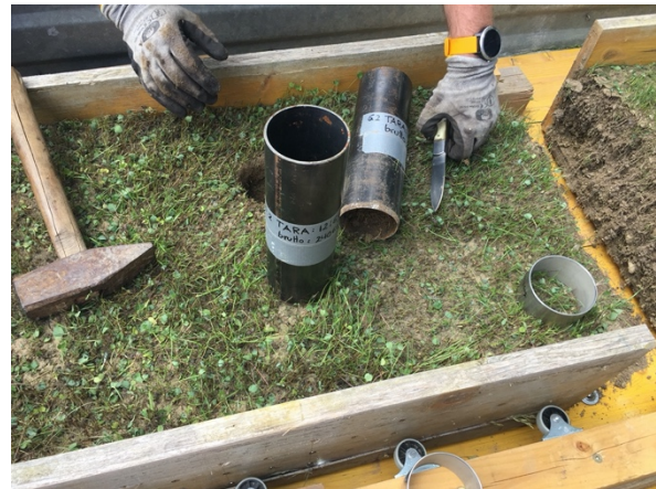
Figure 7. Instrument for measuring pressure Figure 8. Soil sampling for lab analysis
