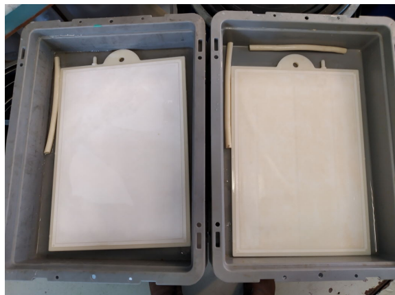
Figure B.9: The polymeric membranes used, before (a) and after (b) cleaning. The left membrane was yet unused.
