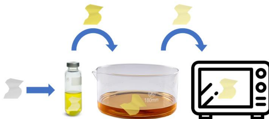
Figure 51 Schematic procedure of the dye modification procedure for the crosslinked PiPOx fibrous mats.
