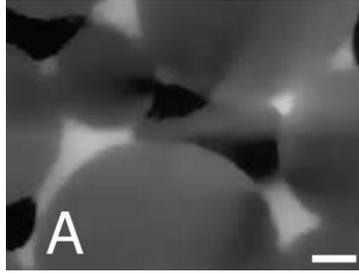
Figure 20: Streakings arising from fluid interfaces moving during a scan. The scale bar is 200  $\mu\text{m}$ .
