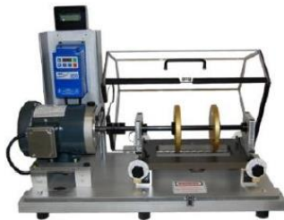
Figure 2: The 'Machinery fault simulator'
