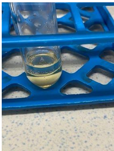
Figure 66: Immiscibility of the produced DES with water
