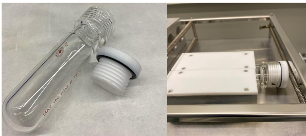
Figure 58: Pressure tube (left) mounted in the aluminum jacket (right)
