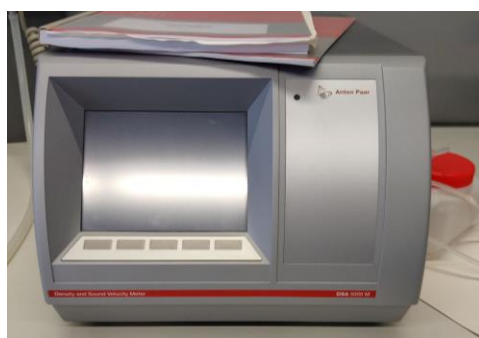
Figure 56: Anton Paar DSA 5000M density and sound velocity meter
