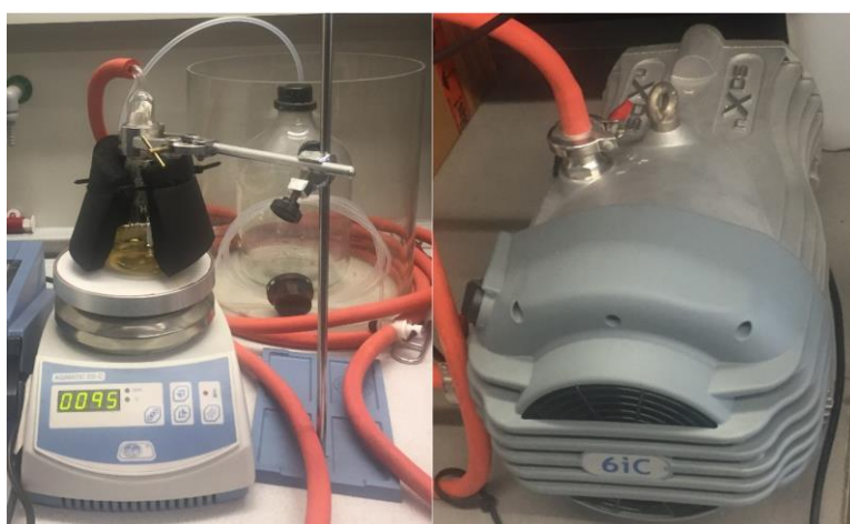
Figure 52: The system used for the vacuum drying; (left) The container and the heating plate and (right) the vacuum pump
