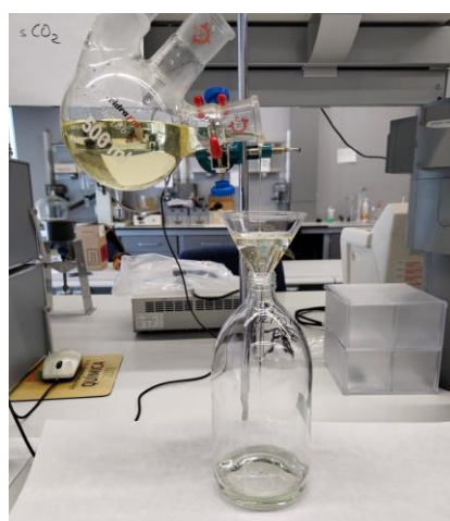
Figure 50: Transferring of the ionic liquid
