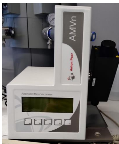
Figure 57: Anton Paar AMVn automatic rolling-ball viscometer
