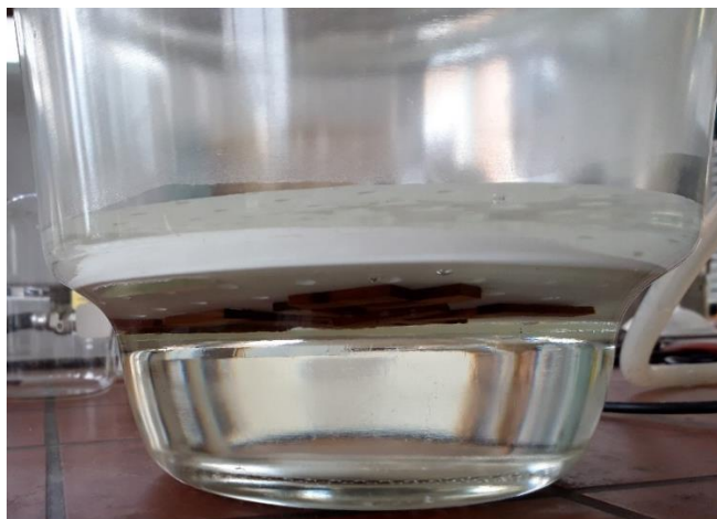
Figure 47: Floating samples of thermally modified spruce after wetting them for a day
