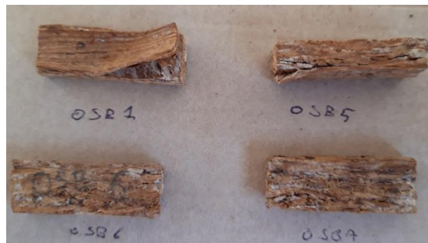
Figure 45: Deterioration of OSB samples caused by C. puteana
