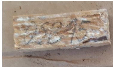
Figure 9: Whitish colour after degradation of OSB due to white-rot fungus
