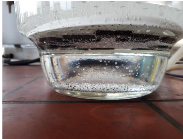
Figure 23: Wetting procedure of porous fibreboard
