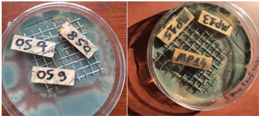
Figure 41: Contamination of OSB (left) and pine plywood (right)
