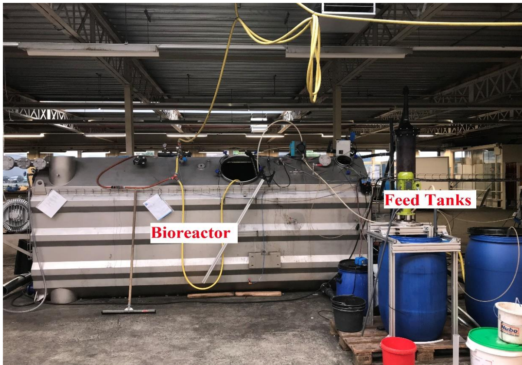
Figure A2.1 - Full-scale Bioreactor in Which the Biofilm Was Cultivated
