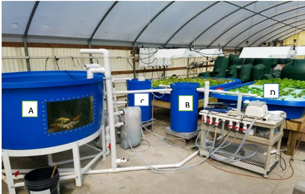
Figure 11. A decoupled aquaponics system design where A is the fish-rearing tank, B is the nutrient sump, C is the digester of mineralization vessel and D is the hydroponic system. Source:astfilters.com
