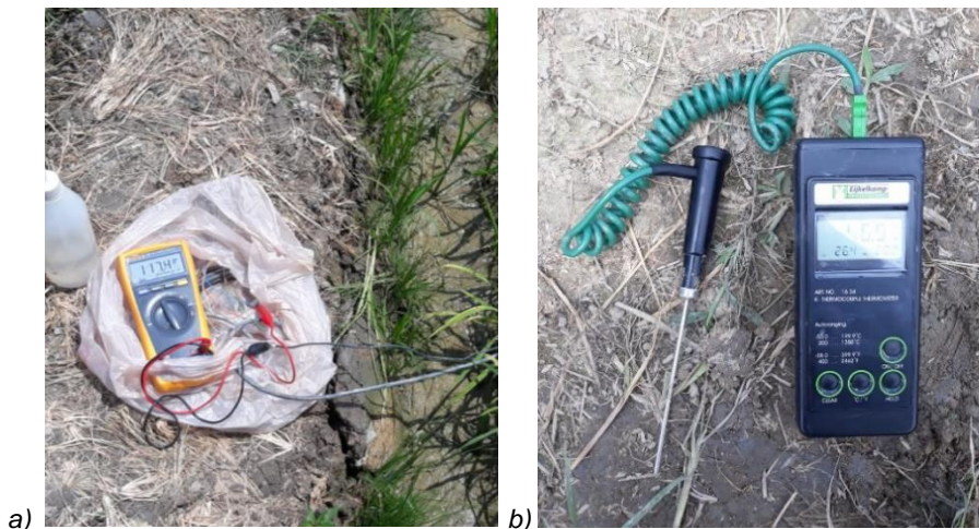
Fig. 12 a) Digital voltmeter with permanently installed Pt-electrode and the Ag/AgCl-reference electrode. b) Thermocouple thermometer for soil temperature measurement.
