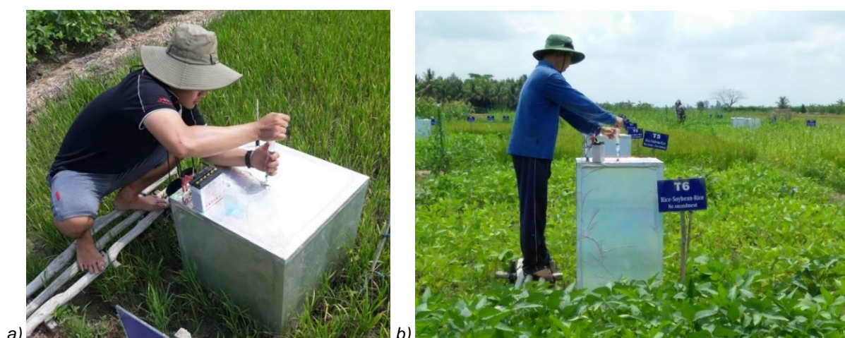
Fig. 14 Gas sampling with a closed chamber and a syringe in a rice plot.
