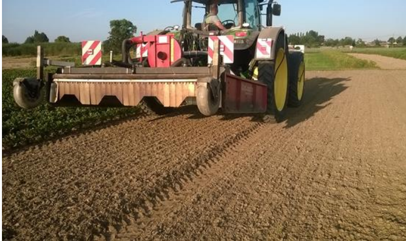
Figuur 3.3 Brander Vanhoucke Machine Engineering T.H.BR. 3000
