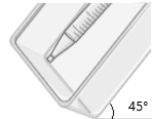
Figure 25. Position of pipette in falcon for rinsing the cell culture with PBS.
