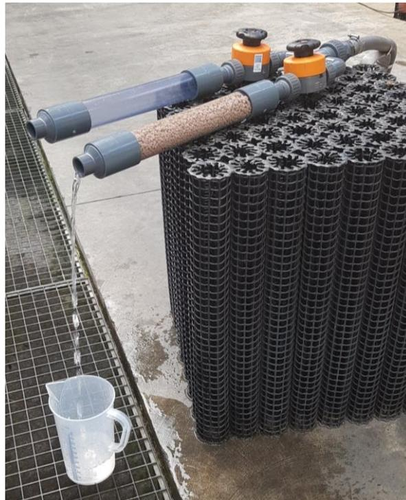
Figure 14. Zeolite filter flow rate measurements
