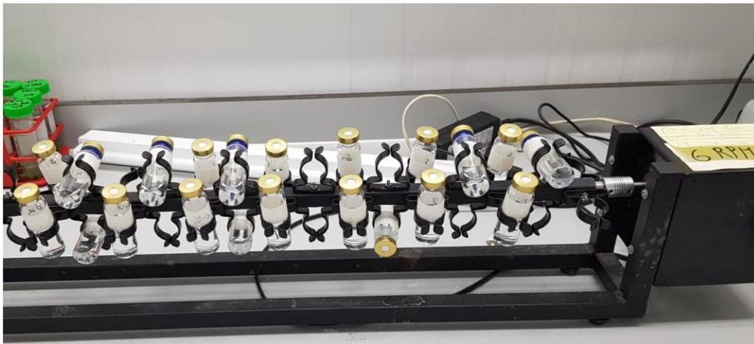
Figure 12. Reactors on rotator.
