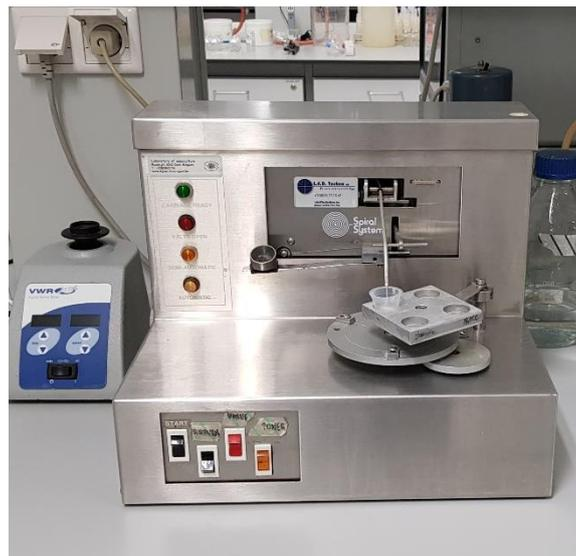
Figure 9. L.E.D Techno Spiral System® Spiral plating machine
