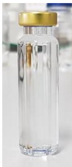
Figure 5. Glass capped vial for geosmin sampling
