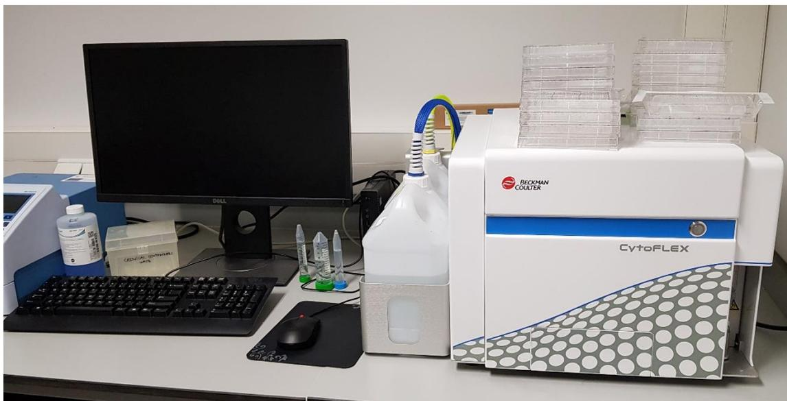
Figure 7. Beckman Coulter CytoFLEX™ flow cytometer
