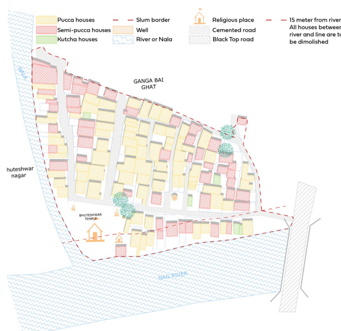
Figure 17. Gujar Nagar Slum. Example of units to be demolished. Based on original drawing received from CFSD
