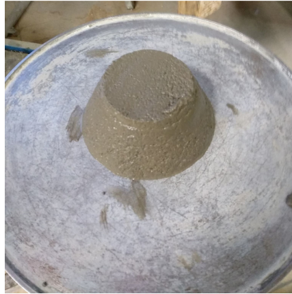
Figure 4-5. Result of flow test for Ca8
