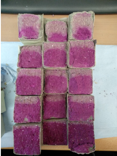
Figure 4-37. Double carbonation front due to yeast extract
