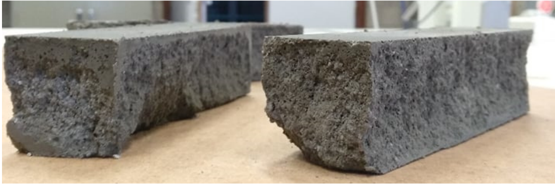
Figure 4-16. Damage to Y2.56 when demoulding after 2 days
