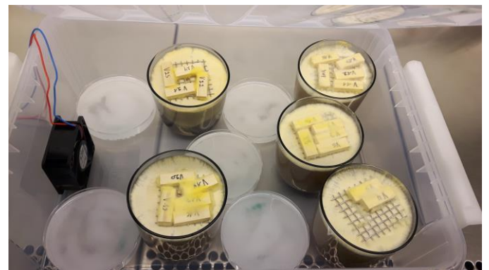
Figure 1: Test setup container for spruce sapwood samples with saturated NaCl-solutions (75% RH) after 6 days of exposure
