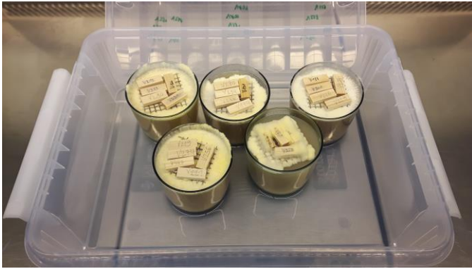
Figure 2: Test setup container for spruce sapwood samples premoistened to 80% MC with demineralized water (100% RH) after 3 days of exposure
