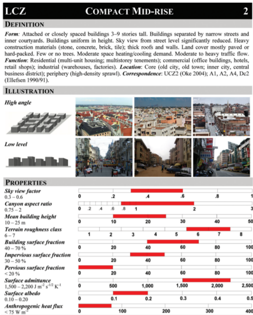
Figure B.1: An overview of the characteristics of LCZ 2, ‘compact mid-rise’ (Stewart and Oke, 2012), one of the key LCZs of Moscow.
