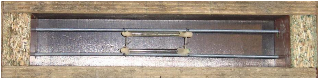
FIGURE 5.1: MOLD PREPARATION FOR A MORTAR PRISM WITH SELF-HEALING PROPERTIES (VAN BELLEGHEM ET AL., 2017B)
