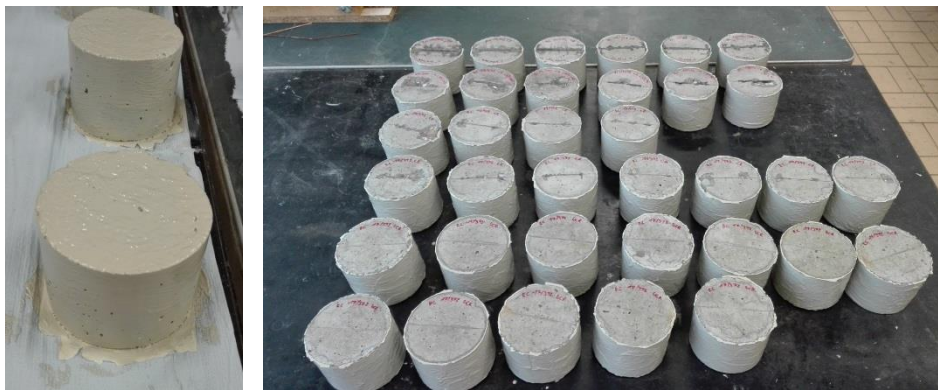
FIGURE 5.5: COATED CONCRETE CYLINDERS (AFTER CRACK CREATION)
