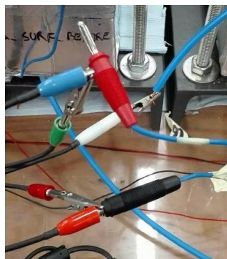
FIGURE 6.17: CABLE CONFIGURATION FOR CONCRETE RESISTANCE MEASUREMENT
