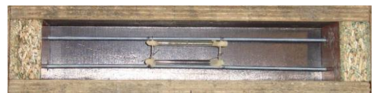
Figure II.1 Mold preparation for a mortar prism with self-healing properties [3]
