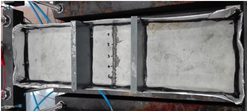
FIGURE 6.8: CRACK HEALING BY MEANS OF CRACK INJECTION, APPLIED ON THE CONCRETE BEAMS
