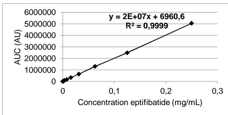
**Figure 4.9: Calibration curve eptifibatide (0.25 mg/mL-0,00012207 mg/mL)**
