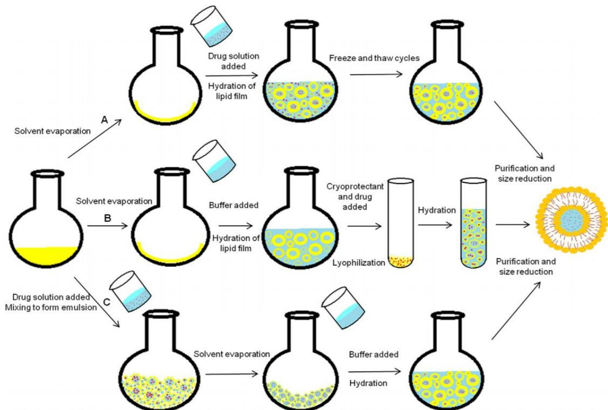
**Figure 1.4: Hydrophilic drug encapsulation by thin-film hydration followed by (A) freeze–thaw cycles, (B) dehydration–rehydration of preformed empty liposomes and (C) reverse-phase evaporation (Eloy, et al. 2014).**
