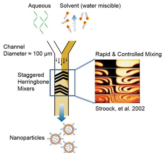
**Figure 1.3: Representation of microfluidic chip for NanoAssemblr™ (Ramsay 2015).**
