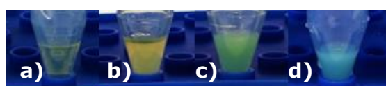
Figure 8.1: Colour development after 4 h incubation at 37°C, a) no activity, b) low activity, c) medium activity and d) high activity
