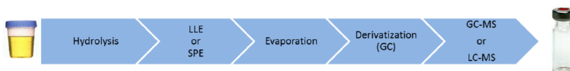
Figure 7: General procedure for sample preparation in doping control [17].
