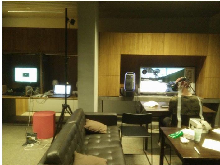
Figure 4: Photo of the experimental set-up with the participants playing the game in the virtual reality condition. The computer on the left provides the oddball task, whereas the laptop in the middle is used to record the EEG and the gaming computer with flat screen on the right provides the game. The subject is seated behind a table to reach the keyboard, response pas and mouse. The table behind the subject carries the EEG recording device and all necessary supplies.
