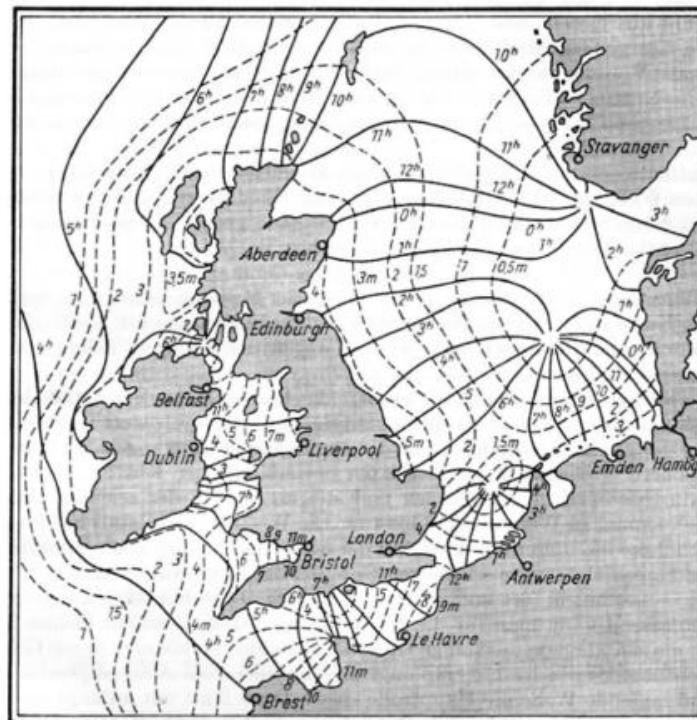
Figure 5. Semidiurnal tides M2 and S2 in the North Sea. Solid lines are co-phased lines (hours) whereas the dashed lines represent the co-range lines (meters) (Pohlmann and Sündermann, 2011)
