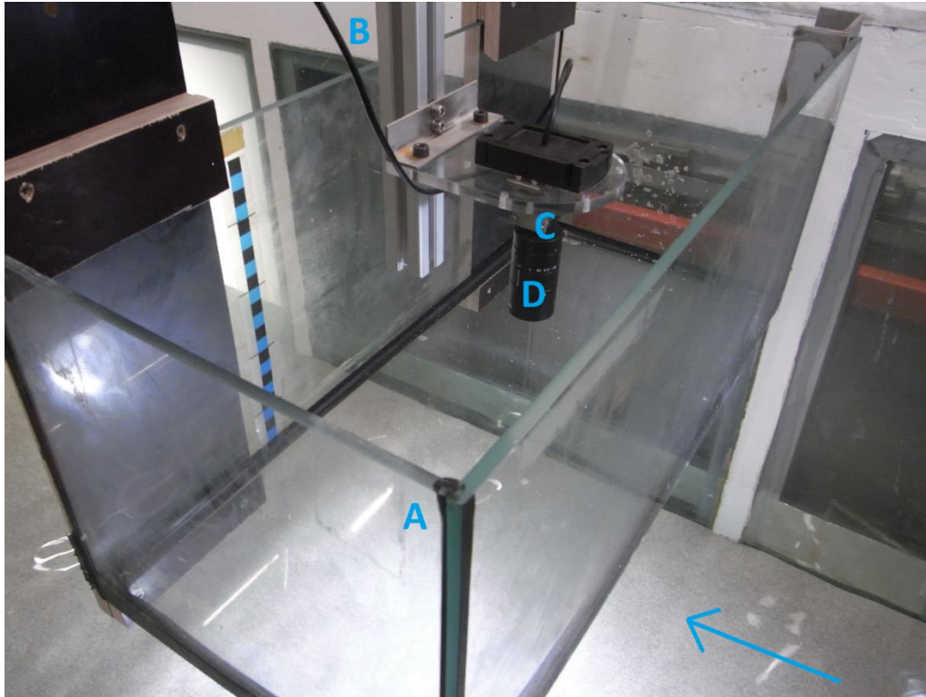
Figure 11: Camera in aquarium above the flume. A: aquarium. B: USB 3 cable to laptop. C: camera. D: lens. Water flow direction indicated by blue arrow
