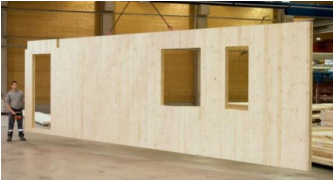
Figure 3 – CLT wall panel with pre-cut openings [7]
