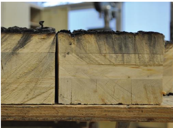
Figure 4 – Charred CLT after fire test [8]
