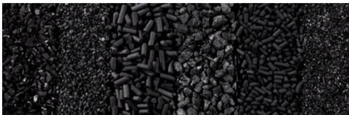
Figure 1.5: Different types of activated carbon delivered by Desotec (Desotec, 2015). The size of the AC from PAC, GAC and extruded AC pellets is respectively around 0.075 mm, 1.65 mm and 4 mm.
